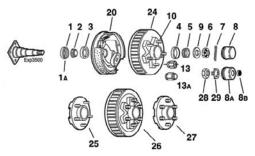
wheels are loose, or spin with a wobble, the bearings must be serviced or replaced.
